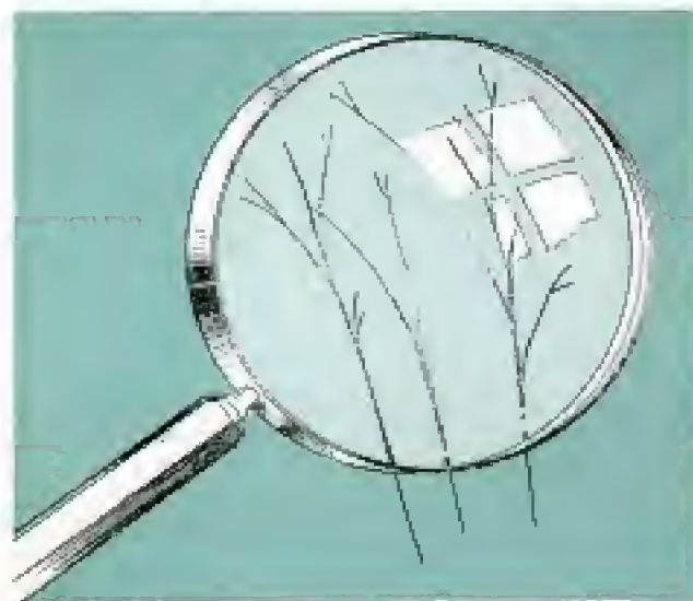
Enlarged view of bristles, below, shows "flags" on good brushes. Flags are visible when brush is held up against light. Brush without flags leaves marks
